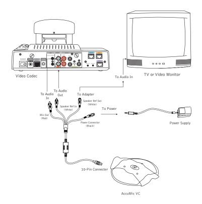
Figure 15. AccuMic VC connections
